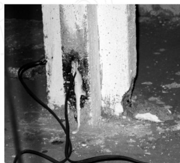
图 8 十字形柱肢端压溃 Fig 8 Compress collapse in end of cross section column
